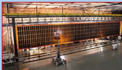
Figure 3: Solar array blanket with mast deployed.
